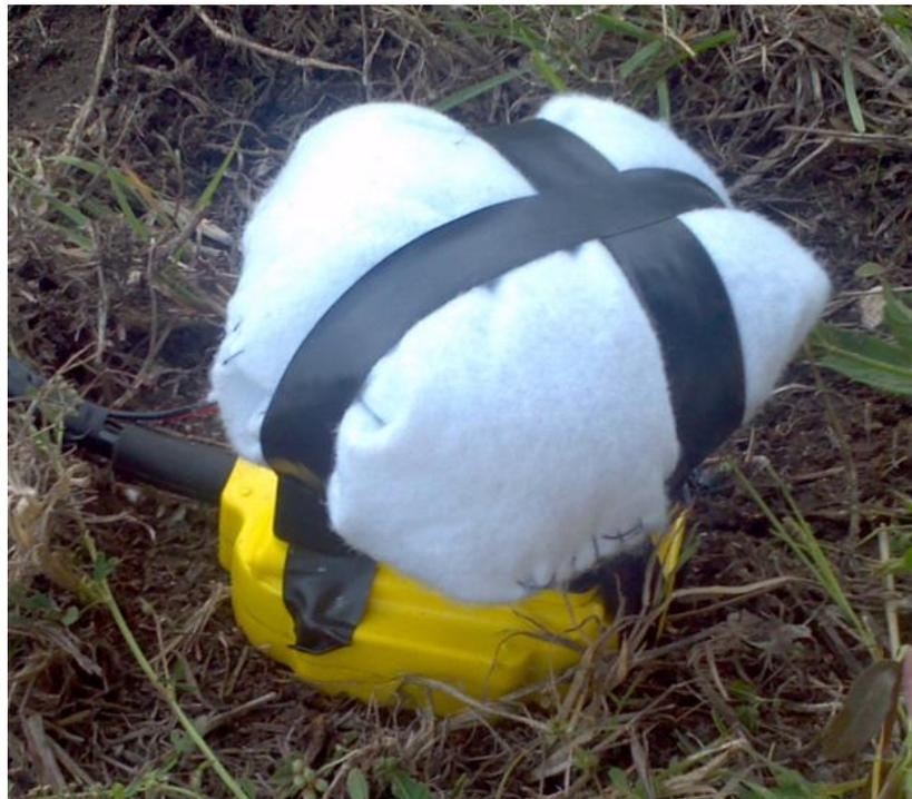
*Figure 3.1: The "pillow-top" vibration isolation system. The piezo microphone is placed inside a felt pocket, surrounded by polyester fibers. These springy fibers dampen vibrations that affect the microphone. Shown attached atop a 3-C geophone.*
