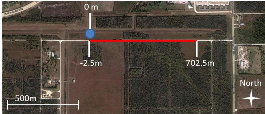
*Figure 3.2: Survey location and schematic. Satellite imagery of the northern portion of the UH Coastal Center, near La Marque, Texas. The blue circle shows the approximate 4-C prototype geophone position, defined as 0 m. The red line indicates the shot line, from -2.5 m to 702.5 m shot at a 5 m interval.*
