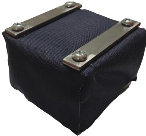
*Figure 3.10: The finished microphone case. The steel plates on top allow the microphone to be stomped on, while the blue nylon keeps the microphone dry.*
