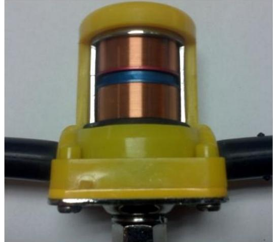
*Figure 1.1: Left: Diagram of a MEMS accelerometer (Hons and Stewart, 2007). As ground accelerations displace the seismic mass there is a capacitance change at the top and bottom electrodes. Right: A cutout analog geophone. The geophone case moves about the seismic mass (copper coils) when subjected to ground motion. The voltage created by the coil is proportional to ground velocity.*
