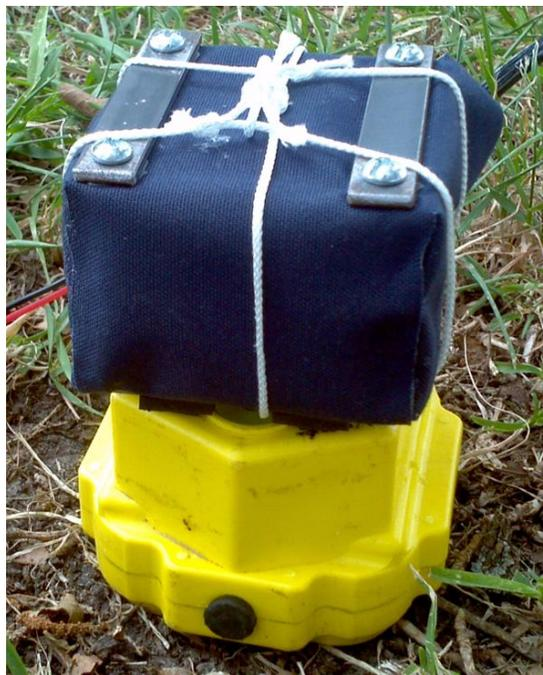
*Figure 3.11: The finished prototype 4-C geophone, sitting atop a 3-C geophone in the field.*
